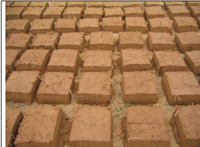
Figure 1: Freshly made adobe bricks drying in the sun
