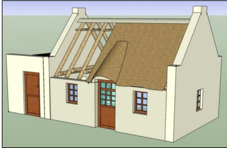
Figure 1: A Scale Model of the Adobe Cottage
